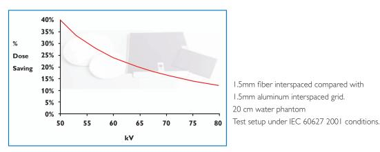
1.5mm fiber interspaced compared with 1.5mm aluminum interspaced grid. 20 cm water phantom
